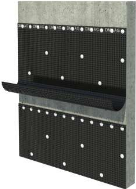
Picture (Above): Horizontal Joint Detail (Picture resembles a portion of the wall.)
