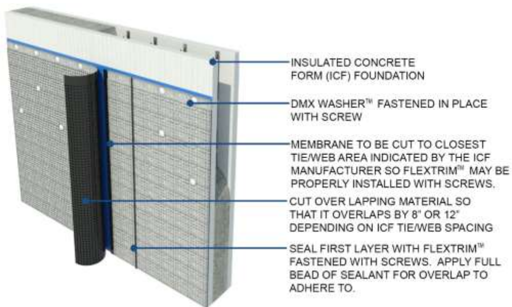
Figure 18 Vertical Joining on ICF
